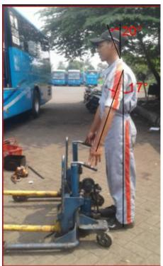
**Figure 8.** Wheel installation with Handtruck *Source: Documentation result, 2018*
