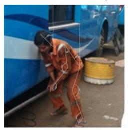
Figure 7. Locking the wheel nut
