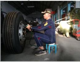
Figure 10. Locking the wheel nut by using chair.
